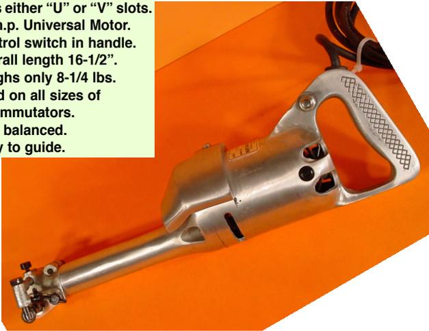
The model K Mica-Miller is an excellent all-around Undercutter for industrial plants or repair shops, as it can be used in the shop or taken to the job, and can be operated on A.C. from any lighting circuit.
