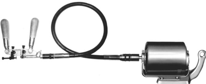
Equipped with Depth Gauge and 2 slot Guides. The angled slot guide is for use on commutators up to 7" diameter. The 1/2" diameter saws allow cutting to within 1/4" of riser.
